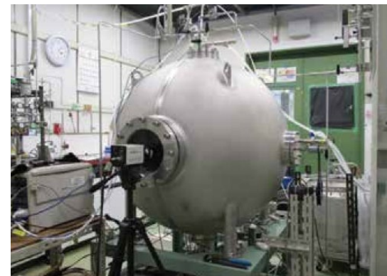
Apparatus to measure flammability limits, essential for safety and risk assessment
