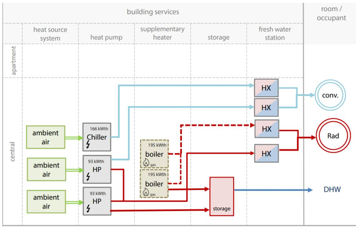
Multiple (cascade) centralized HP system with back-up boiler and chiller for AC
