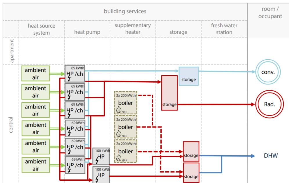
Multiple centralized HP systems and booster HPs for Air Conditioning (AC) with back-up boiler
