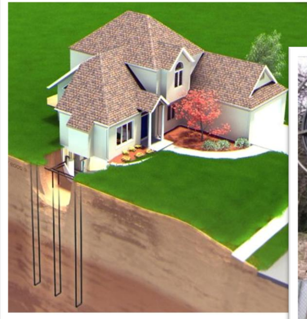
Vertical Borehole Heat Exchangers (BHEs)
