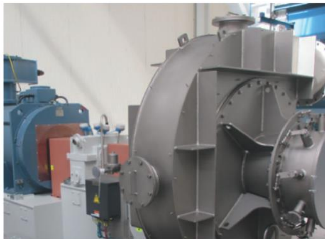
Figure 1: left: PILLER High Performance Blower, right: Multi-stage system in operation
