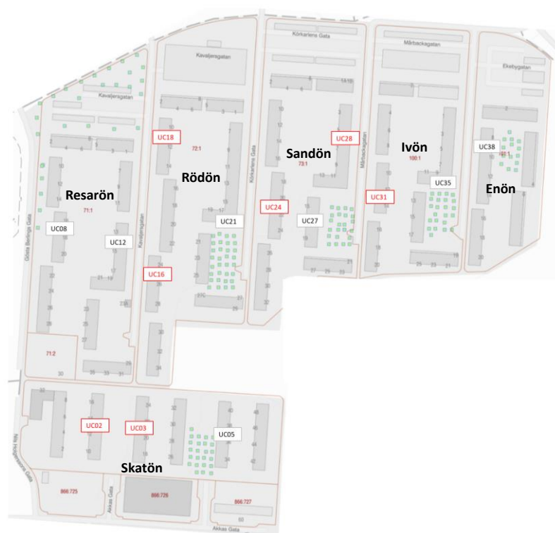
Figure 2 Overview of Backadalen multifamily building complex including the location of the 146 boreholes in the Borehole Energy System
