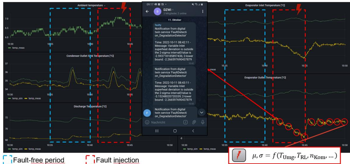
Figure 1: First results of fault detection service for evaporator fouling and resulting user notification.
