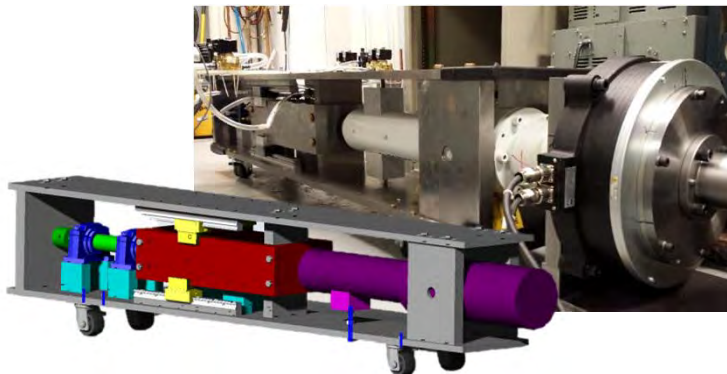
GEN-2: compression based 140 W water cooling (2014)
