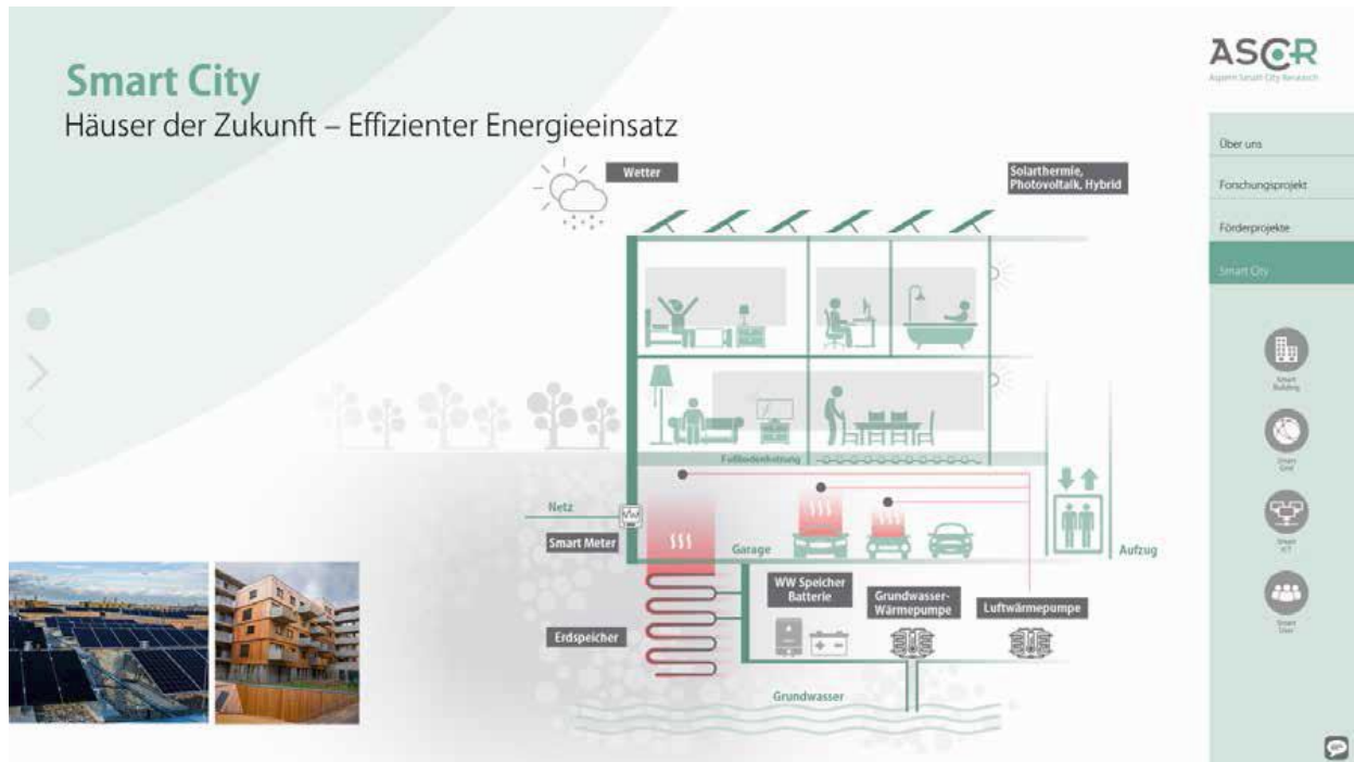
Figure 51: Schematic diagram of the heating system in the Smart City Aspern (Niederbrucker et al., 2016)
