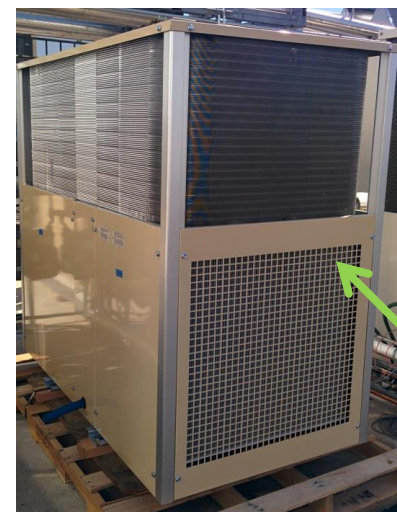
Engine & compressor compartment
