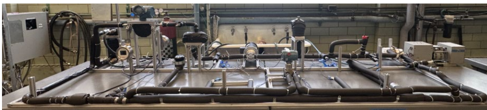
Figure 3: A3-certified two-phased pumped loop for composition shift and heat transfer measurements, located at the Ray W. Herrick Laboratories
