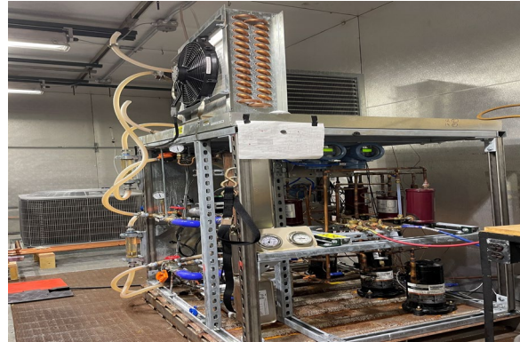
Figure 2: Propane cold climate heat pump situated in A3 psychrometric chambers at the Ray W. Herrick Laboratories
