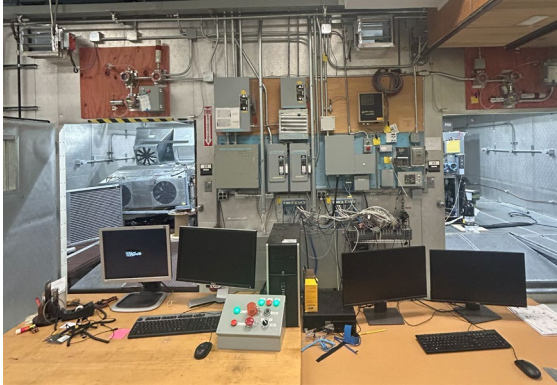
Figure 1: Pair of A3-certified psychrometric chambers at the Ray W. Herrick Laboratories
