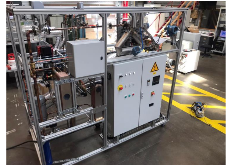
Test bench for testing two-phase scroll compressors (H2020 Regen-by-2 project)
