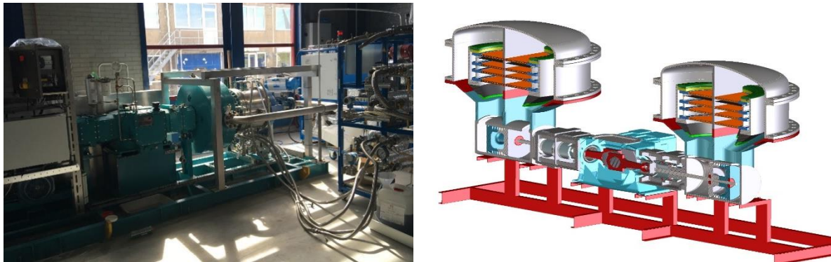
Figure 4-46: COMTA bench scale thermoacoustic heat pump (left) and artist impression of a two piston double acting industrial TAHP (right).
