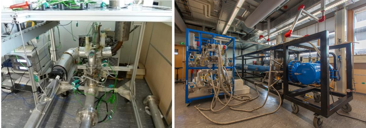
Figure 4-40: Thermoacoustic heat engine (left) and compressor driven thermoacoustic heat pump (right) tested in Catch-IT.
