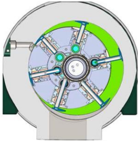
Figure 4-48: Cross-sectional view of the TC-C920 rotary vane compressor.
