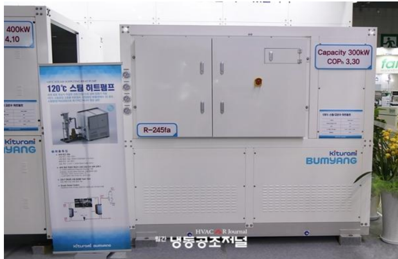
Figure 4-60 Bumyang's steam generation heat pump at 2019 HARFKO (Source: https://www.hvacrj.co.kr/news/articleView.html?idxno=10287 ).
