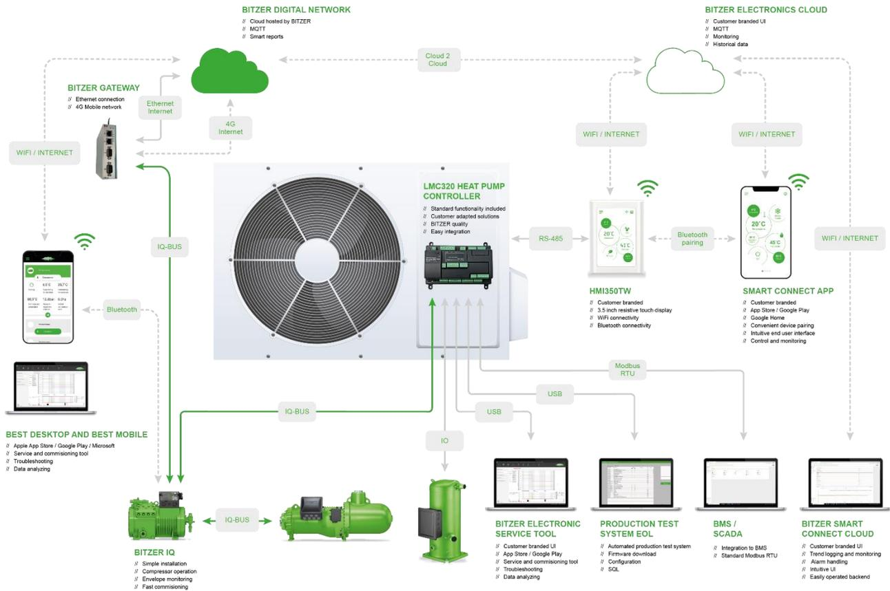
Figure 1: Overview of the Bitzer Heat Pump Ecosystem
