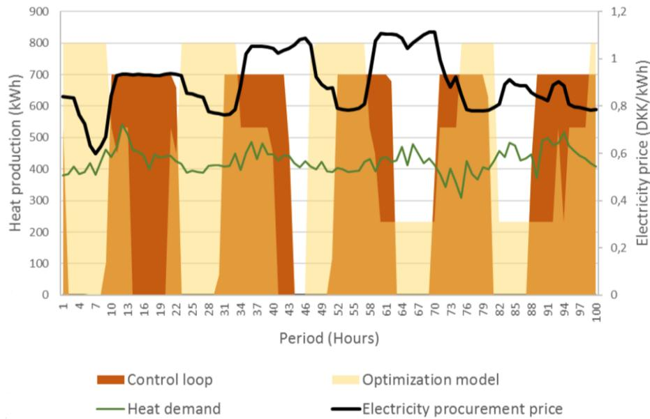
**Figure 2: Flexible heat production during winter [HOFOR, 2021]**
