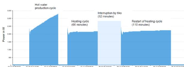
**Figure 2: heat pump cycle interrupted by tiko control [1]**
