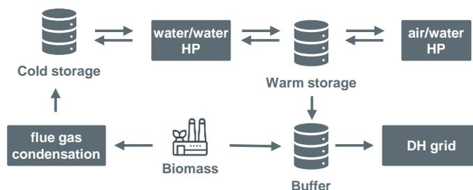
In summer, the biomass plant is not operational and the heat from flue gas condensation is replaced by air-water heat pumps which deliver heat at level of 30/35°C that was done by the flue gas condensation before. From there on, same procedure as in winter. Heat load in summer is around 0.5-1MW.
