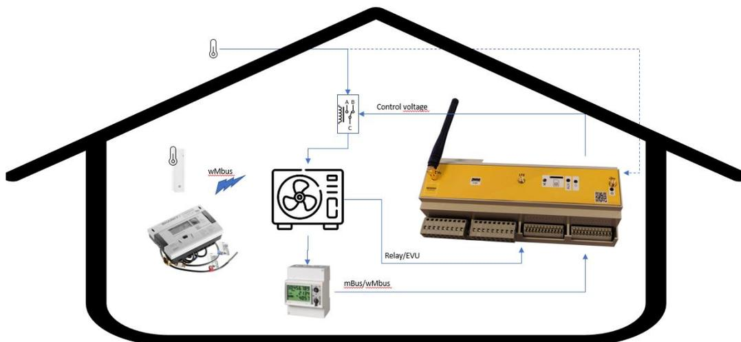
**Figure 1: Hardware setup for PreHEAT Heat Pump Controller.**
