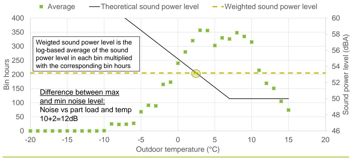
Proposed test point for sound power test: +2°C, 54% (test point B in EN14825), for air source heat pumps +7°C, but part load according to test point B (54%)
