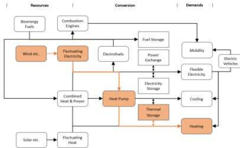
Figure 2: Operation of a Smart Energy System when there is integration of wind power.
