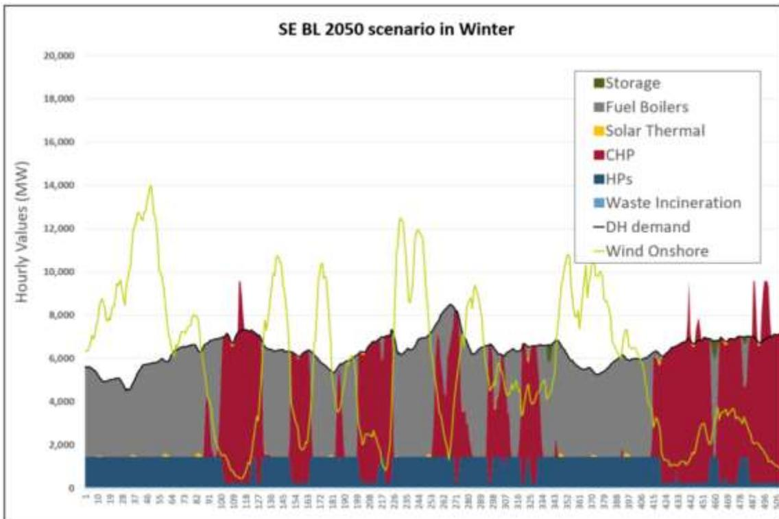
Figure 17: CHP and large-scale HPs heat production, onshore wind power and DH demand during the first hours of the year in the SE BL 2050 scenario (Source HRE4 project)
