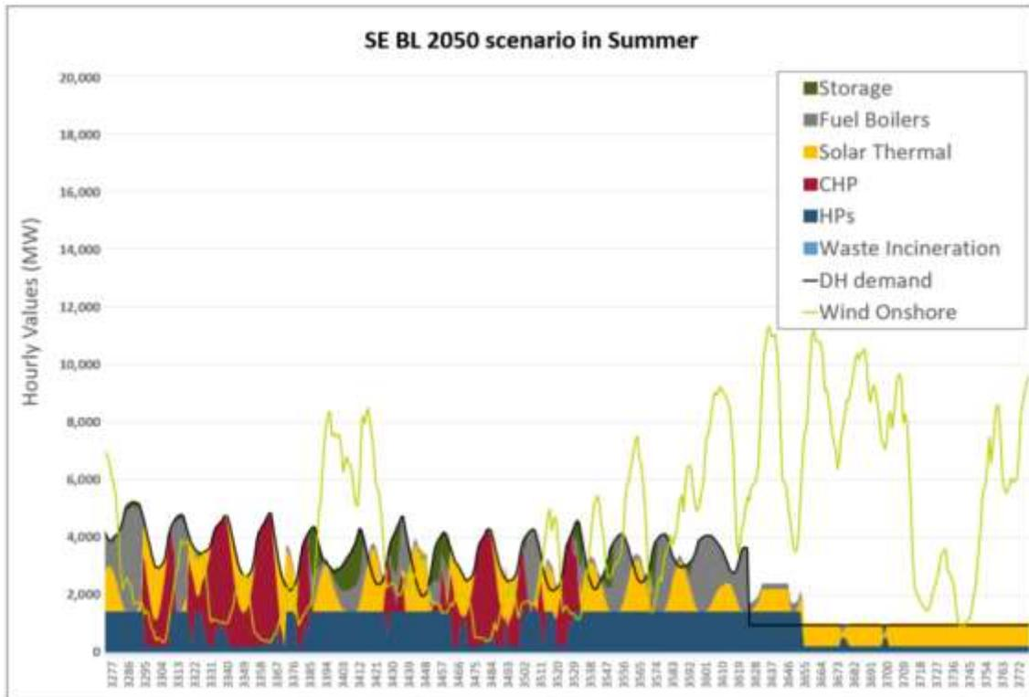
Figure 19: CHP and large-scale HPs heat production, onshore wind power and DH demand between the middle of April and the middle of May 2050 in the SE BL 2050 scenario (Source HRE4 project)
