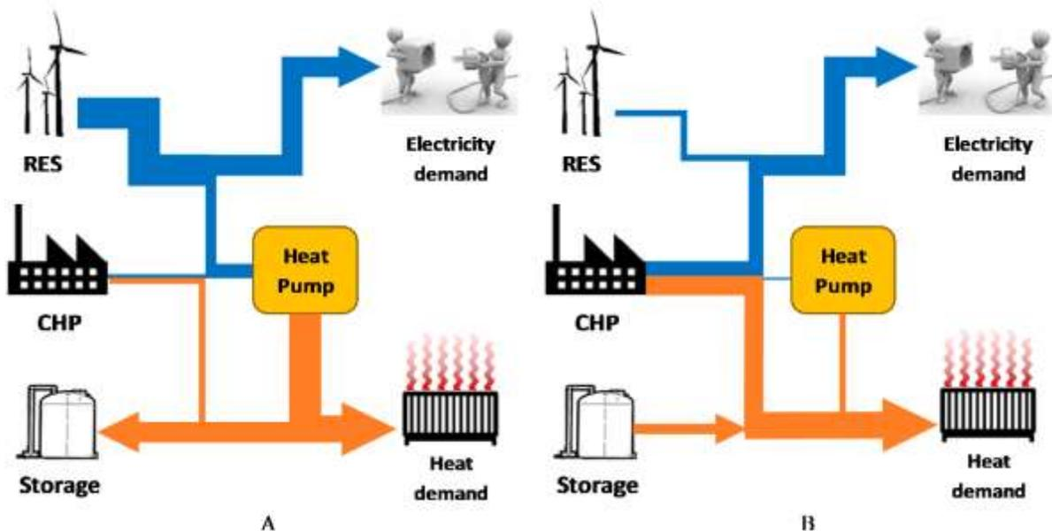
Figure 10: Large-Scale HPs used with high share of RES (A) and HPs used with low share of RES (B) [2].
