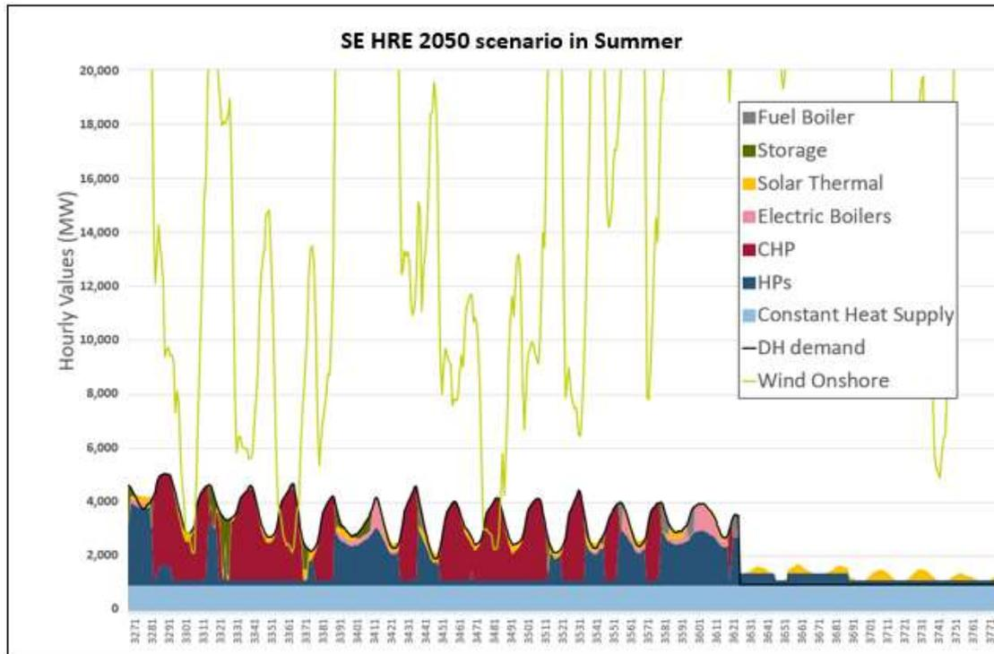
Figure 18: CHP and large-scale HPs heat production, onshore wind power and DH demand between the middle of April and the middle of May 2050 in the SE HRE 2050 scenario (Source HRE4 project)
