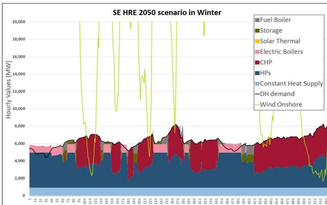
Figure 16: CHP and large-scale HPs heat production, onshore wind power and DH demand during the first hours of the year in the SE HRE 2050 scenario (Source HRE4 project)
