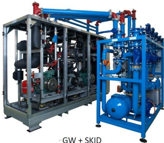
Reduses heat pump is delivered as a skid installed and tested at the factory to be able to install plug & play
